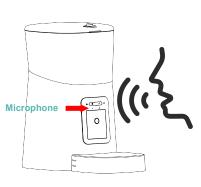
3. After recording is complete, the feeder will play a preview of the recorded audio. If you need to change the recording, please re-record it. The default voice recording playback is 3 times.
