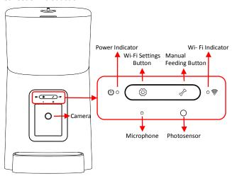
5. You can push the camera to turn down to observe the feeding tray. The feeder supports up to 4 levels of angle adjustment. It supports Micro-SD card recording, and the SD card slot is visible when the camera is turned to the bottom.
